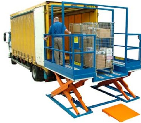
Functionality and practicality have been successfully combined with safety. The Pitfree MultiDock is the only Loading Bay Lift with twin operator safety zones which encapsulate the operator in a steel safety frame to protect him from falls and crushing which are the two main causes of injury in the Loading Bay.
